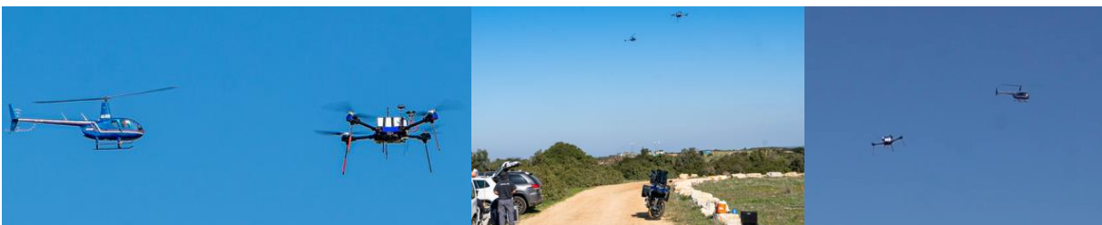
A drone and a helicopter equipped with C&CAS; C&CAS flight test, Jan. 18 th 2023, Israel. The C&CAS automatically steers the drone away whenever the drone is risking the helicopter.
